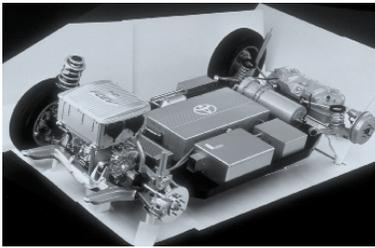
Toyota's fuel cell RAV4 employs a 25-kilowatt fuel cell that works in conjunction with a downsized electric vehicle battery pack. The batteries are constantly recharged
