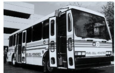
the Department of Energy. In 1994 and 1995, Georgetown rolled out three 30-foot buses that were the world's first fuel cell vehicles capable of operating on liquid fuels. In 1998, Georgetown will unveil two methanol-fueled prototype 40-foot transit buses using two different fuel cell technologies. International Fuel Cells has provided
